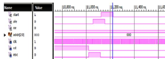
Figure 2: Simulation – ADC Controller module
