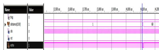
Figure 3: Simulation – Ultrasonic Controller module
