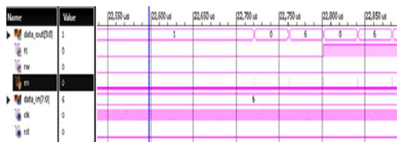
Figure 4: Simulation – LCD Controller Module
