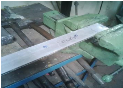
Fig. 12. Specimen held as cantilever beam
